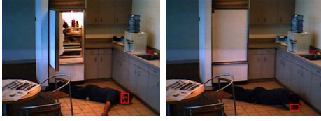
Figure 4. Two examples of head detection using skin color. Note that in the example on the left, the mask has ruled out the refrigerator door as non-human event and correctly identified the human body as the human object.
